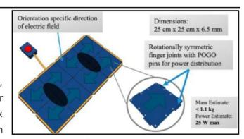
Electrodynamic Dust Shielding (EDS) system to mitigate lunar dust in a variety of applications.
