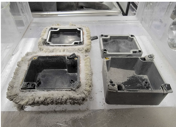
(21) Boxes after failed seal test
